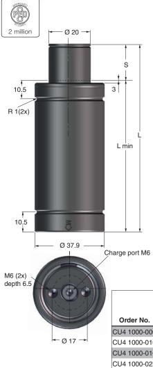
The CU4 gas spring is a very compact Bore Sealed gas spring with impressive force in a compact body. The maximum frequency for the spring is 100 strokes/ minute.
